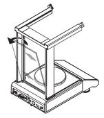
Push the lock button to release the rear glass.
